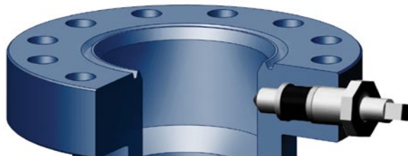
Optional C22-BP has lockscrews to hold the wear bushing in place.
